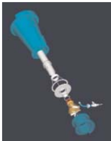
Schematic diagrams of components of the Precision Granulator™
