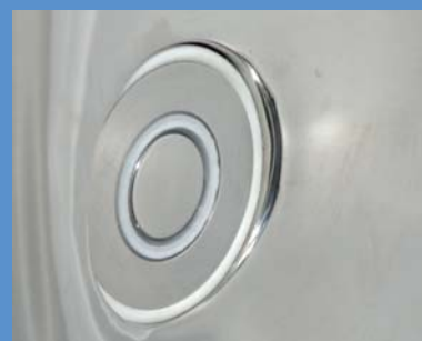
CIP position at end of process The probe is completely retracted to enable complete cleaning of wash chamber and seal.
