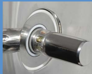
In process measurement position The probe is inserted into product ready to take multipoint measurement.
