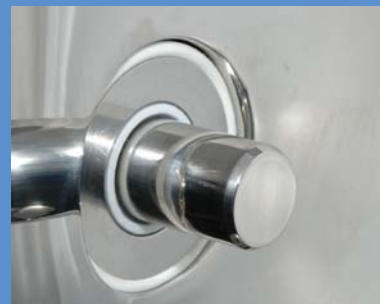
Clean and calibrate position The probe is retracted in order to clean window and check calibration.
