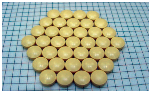
Figure 3: Coated tablet appearance (10% weight gain)
