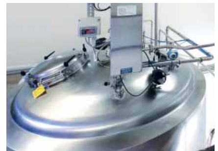
The Niro Pharma Test Station includes a validated purified water production and distribution system. The PW production unit supplies the spray dryer CIP and feed systems with water meeting the pharmacopoeial quality standard.
