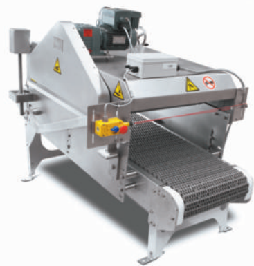
The Bag Flattener, mounted above the bag conveyor, prepares the bag for stable palletising by means of powered rollers.
